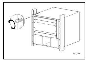
2 Slide the guide onto the loosened screws.
